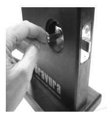
→3) Insert the spindle into the latch mechanism while depressing the button. The spindle is properly installed when the button pops-up on the opposite side of the latch, and the spindle is locked into place.
